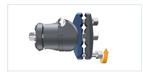
Position the spring over the middle bolt of the Pin Clamp and place the pin head on top. Depress the spring until the pin clamp head has come into contact with the opposite side.
