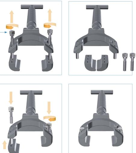
For assembly place the clamp fixation blocks with the lip oriented towards the inside of the Reduction Handle over the pins and hand-tighten the bolts from the opposite side.
