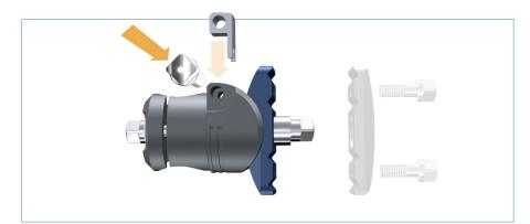
Place the pin clamp insert into the dedicated opening at the pin clamp socket and seat the bolt back into the socket.
