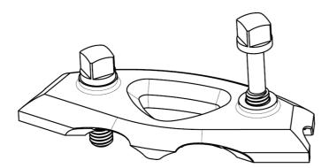
2. Add the second coupler flange and tighten it with the two tightening screws.
