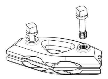
2. Separate the two coupling halves and the coupling is now ready to be cleaned.
