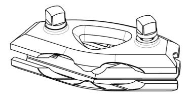
3. Untighten the screws 1-2 turns to ensure, that Ø11mm connecting rods fit into the rod coupler.
