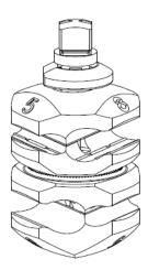
3. Release the coupling. The screw head must fit within the washer. Turn the screw 90° clockwise to prevent screw jamming during storage. The coupling is now assembled.
