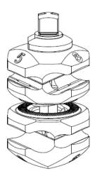
2. Align the slot in the washer with markings at screw head. These markings are an indicator for the position of two notches on the screw shaft which allow removal of washer only at this specific alignment.
