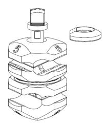
5. Release the coupling. The coupling is now ready to be cleaned.
