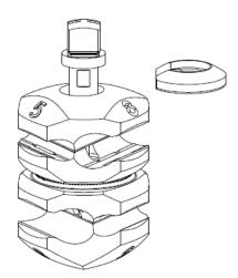
2. Insert the washer. Insertion of washer is only possible at the level of notches on the screw shaft.
