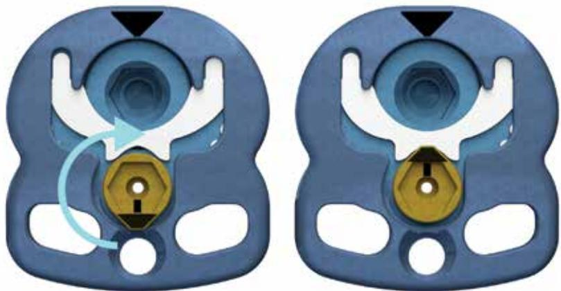
**Figure 27.** Locking the Plate
